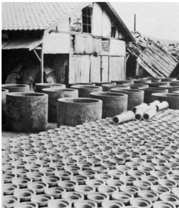
CEMENT DONATED BY UNCACK was used to make well casings and pipe, July 1952.
