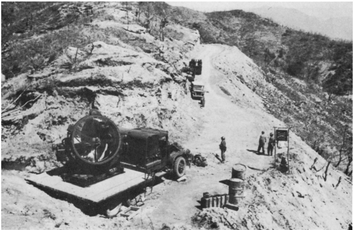
SEARCHLIGHT IN POSITION, west of Ch'orwon. This searchlight is mounted on the bed of a converted 2 \frac{1}{2} -ton truck.
